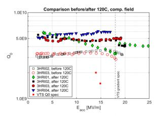
Figure 2: Q vs E performance in VTS for the four design verification cavities before and after 120C bake.
