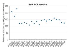
Figure 4: Bulk BCP removal by weight, cavities in chronological order of surface treatment.
