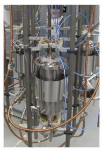
Figure 5: Three 3.9 GHz cavities assembled to the insert, ready for testing in VTS.
