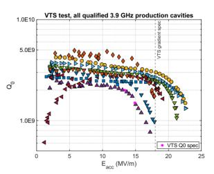
Figure 6:  $Q_0$  vs E performance for all cavities that were accepted for string assembly.
