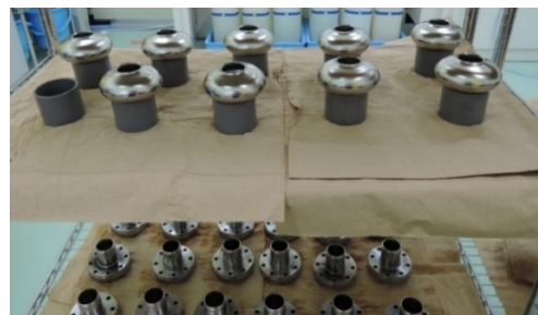
Figure 11: A picture of the NbTi flanges and Nb parts which were being dried after BCP and pure water rinsing processes in a clean room at KEK.
