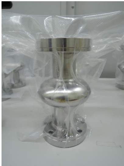
Figure 12: A picture of packed NbTi flanges and Nb parts for a cavity at KEK.
