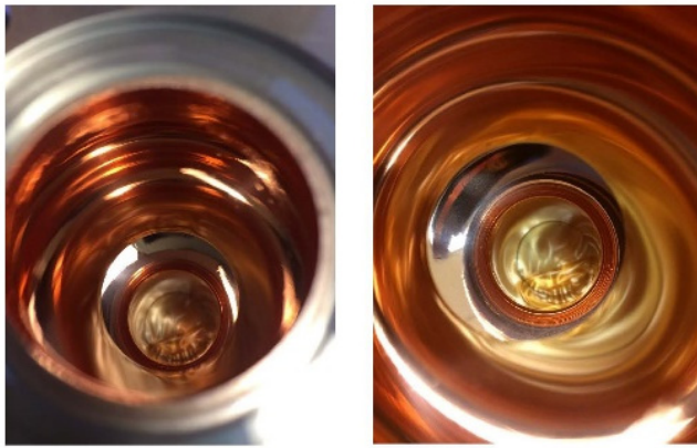
Figure 7: Pictures of inner-surface of 3.0-GHz single-cell Cu cavities after CBP process at JLab.
