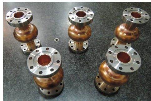
Figure 5: A picture of 3.0-GHz single-cell Cu cavities which were assembled at KEK.
