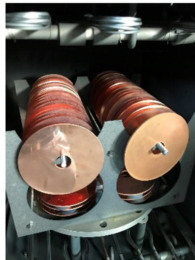
Figure 1: A picture of Cu (C1020) disks set in the vacuum furnace for annealing process.
