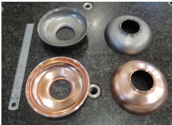
Figure 3: A picture of trimmed Cu and Nb cups.
