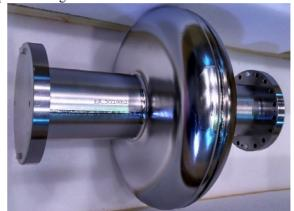
Figure 3: PIP-II LG002 single-cell.
