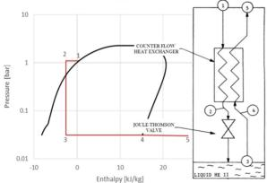
Figure 7: Conceptual layout of the 2 K refilling system for the LASA facility and corresponding points in the pressure-enthalpy graph of helium [9].
