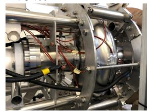
Figure 4: PIP-II FG001 single-cell during preliminary EP treatment at E. Zanon.
