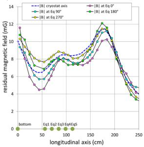
Figure 6: Measurement of the vector amplitude of residual magnetic field in the vertical cryostat at LASA. Horizontal axis starts at cryostat bottom, green dots visually report the heights of each cavity equator.
