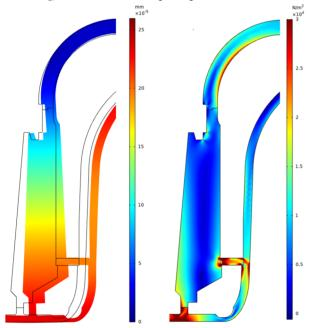
Figure 2: FEM analysis (strain on the right, VM stress on the left) of the spool transition ring while withstanding the reaction force of 10 MV/m cavity field. Peak values in the colour code are 0.25 µm and 0.03 MPa, respectively.
