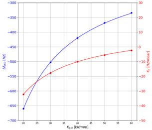
Figure 1: LFD frequency shift (blue) and pressure coefficient (red) as a function of external cavity stiffness for a cold cavity.
