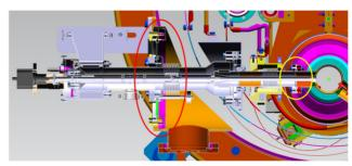
Figure 2: Section of an EXFEL coupler assembled in the cryomodule; in red and yellow the connections to the module (fixed points).
