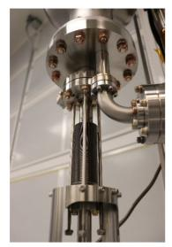
Figure 2: The movable coupler assembly is screwed on a 2.75" Conflat, screwed to a 6" diameter SS flange compatible with XFEL/LCLS-II beamline cavity flanges.
