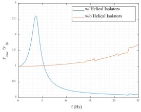
Figure 9: FRF of the lateral displacement of the reference cavity – With and without helical isolators.
