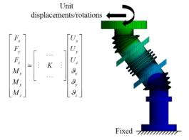
Figure 3: Equivalent stiffness matrix computation.
