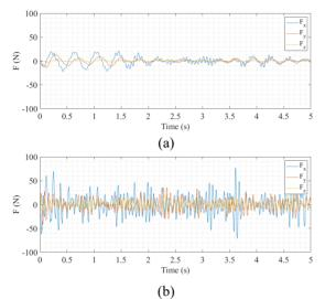
Figure 10: Force on a reference bellows -a) TT equipped with helical isolators; b) rigid TT.
