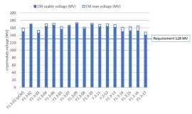
Figure 3: Cryomodule Voltage Gain.
