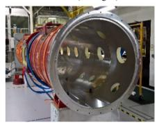
Figure 7: Magnetic shield inside the vacuum vessel.
