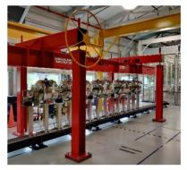
Figure 6: String assembly under the lifting tooling.
