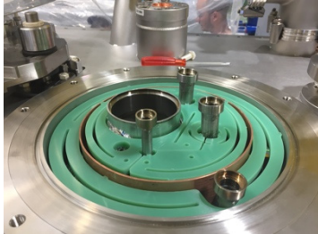
Figure 10: Jumper centering part on cryomodule.
