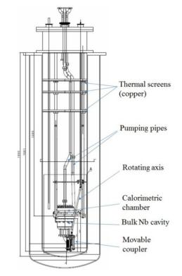
Figure 2: Drawing of the cavity mounted inside the cryostat with movable coupler.
