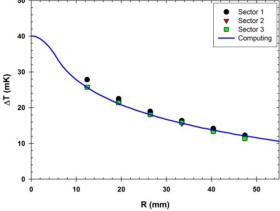
Figure 4: Temperature variation profile along radius of sample. The theoretical curve has been obtained from AN-SYS calculation with following parameters: Pstat=12.5 mW, e=2.2 mm,  $h_k$ = 900 W/m<sup>2</sup>K. The thermal conductivity has taken from experimental measurements.
