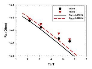
Figure 8: Surface resistance measured with the thermometer T110 at B≃1mT for 4.3 K, 3.0 K, 2.0 K and 1.65 K. Straight lines are the theoretical R<sub>BCS</sub>.
