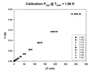
Figure 3: Calibration curves for the 9 outer thermometers. The temperature variation is strongly dependent of the exchange coefficient (surface roughness and Kapitza conductance à Nb/He(II) interface).
