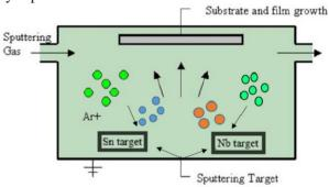
Figure 1: Schematic diagram of the principle of magnetron sputtering.
