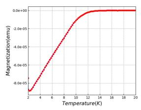
Figure 2: MPMS image of Nb3Sn film.
