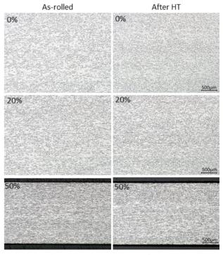
Figure 10: Microstructure in the plane formed by the short transverse and rolling directions for as received sheet (0%) and 20% and 50% thickness reductions, before and after HT. Original magnification 100x.
