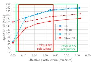
Figure 12:  $Rp_{0.2}$  and  $R_m$  vs. effective plastic strain, before and after HT. Rectangle boxes contain the range of effective plastic strains in 75 and 90% of RFD pole surface respectively. The graph is similar to Fig. 8, but x-axis has been replaced by effective plastic strain.
