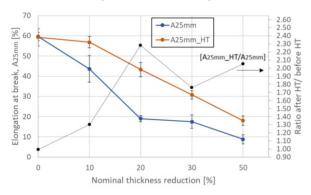
Figure 9: Overview of the  $A_{25mm}$  values before and after HT in function of the thickness reduction achieved by crossrolling. Error bars represent one standard deviation. Secondary axis indicates the ratio (after HT/before HT).
