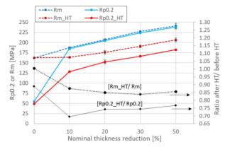
Figure 8: Overview of the  $R_m$  and  $Rp_{0.2}$  values before and after HT vs. thickness reduction by cross-rolling. Error bars represent one standard deviation (note that deviations are very low, indicating high repeatability). Secondary axis indicates the ratio (after HT/before HT).
