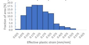
Figure 2: Histogram of the percentage of the RFD Pole surface having seen certain level of effective plastic strain.
