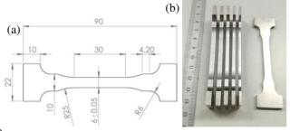
Figure 6: a) Tensile specimen drawing. b) Ready-to-test specimens of different thickness, from left to right: 0, 10, 20, 30 and 50 % thickness reductions.
