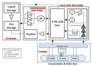
Figure 2: Schema of cryogenic refrigerator configuration.
