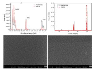
Figure 2: (Top left) XPS data indicating the sample of NbTiN deposited on Nb is niobium-rich while the layer deposited over AlN is N-rich. (Top right) XRD data showing shifted diffraction peaks between the two NbTiN samples. (Bottom left) SEM image of NbTiN on AlN. (Bottom right) SEM image of NbTiN on Nb.
