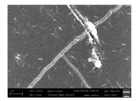
Figure 4: SEM image taken on 800 nm thick MgB<sub>2</sub>.
