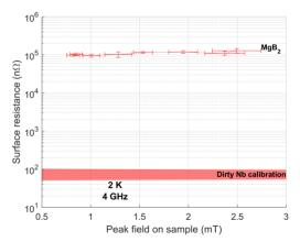
Figure 5: Measured surface resistance of 400 nm thick MgB<sub>2</sub> at 4 GHz and 2.0 K. Error bars do not include a large systematic error resulting from mismatch between extra dissipation in calibration and sample measurements [1].
