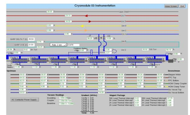
Figure 3: LCLS-II cryomodule EPICS cryo-control controls. Showing valves, heaters and temperature sensors.
