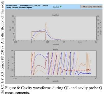
Figure 6: Cavity waveforms during QL and cavity probe Q measurements.
