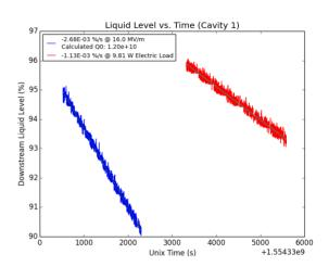
Figure 5: Qo Measurement: He Liquid level vs. electric heat and RF heat.
