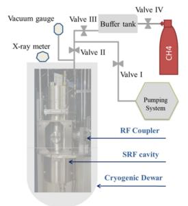
Figure 1: schematic diagram of experiment for cryogenic adsorption.
