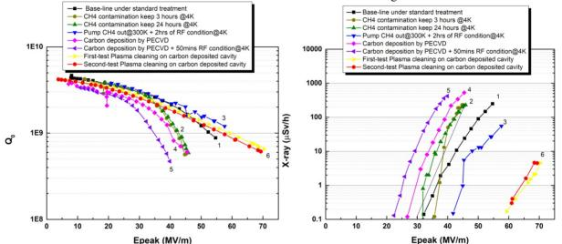
Figure 2: Experiment results under different surface treatment, the left and right was the dependence of Q0 value and X ray radiation dose on the surface peak electric field, respectively.
