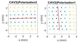
Figure 5: Normalized amplitude of Polarization2 (left) and Polarization1 (right) at cavity three in ACC2 as a function of the beam position. The red lines indicate the fitted polarization axes.
