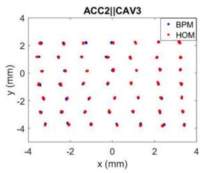
Figure 4: Calibrated beam positions (red) and the BPM interpolated positions (blue) in cavity three in ACC2.
