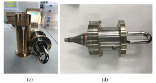
Figure 3: (a) Detachable parts, (b) T type inner conductor, (c) the fixture used for installation, (d) HOM coupler prototype.
