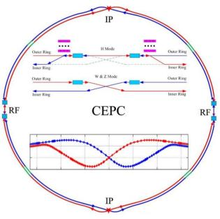
Figure 1: Layout of CEPC collider.
