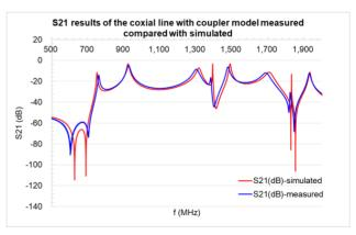
Figure 10: The measured S21 parameters of the HOM coupler compared with simulated.
