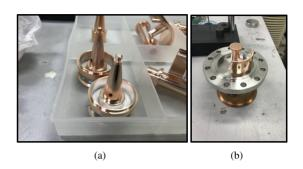
Figure 4: (a) The ceramic window, (b) the upper part of the HOM coupler .
