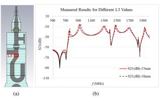
Figure 13: (a) HOM coupler model, (b) measured results for different L3 length.
