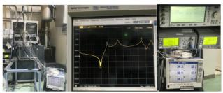
Figure 14: High power test for the HOM coupler at room temperature.
