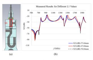
Figure 11: (a) HOM coupler model, (b) measured results for different L1 length.
