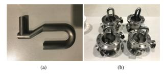
Figure 5: (a) The loop part, (b) the bottom part of the HOM coupler with helium jacket.
