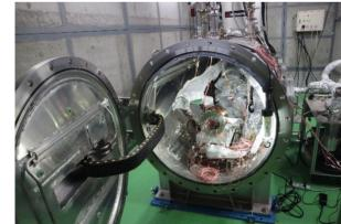
$\frac{3}{2}$  Figure 7: The prototype HOM absorber was installed in  $\frac{3}{2}$  the horizontal cryostat.
