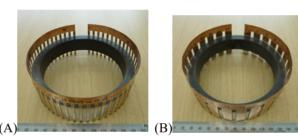
Figure 4: Test pieces which brazed an AlN cylinder and thin copper strips. The width of a copper strip is 3 mm for test piece (A) and 10 mm for test piece (B).
