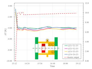
Figure 8: Heat removal test results of the new prototype HOM absorber.
