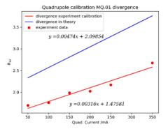
Figure 5: Quadrupole focus and defocus strength calibration.
