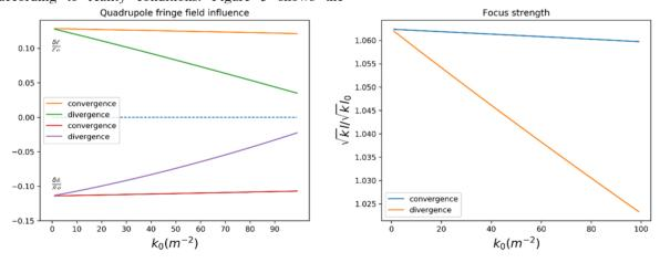
Figure 4: Quadrupole fringe field effects. In left figure  $\frac{\delta l}{l_0} = \frac{l_f - l_0}{l_0}$  or  $\frac{l_d - l_0}{l_0}$  and  $\frac{\delta k}{k_0} = \frac{k_f - k_0}{k_0}$  or  $\frac{k_d - k_0}{k_0}$ .
