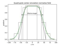
Figure 2: Quadrupole center magnetic field gradient
