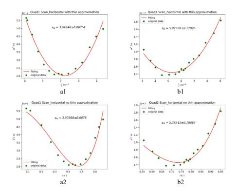
Figure 3: Emittance results. a1 and b1 are fitted using Eq. (7) and a2 and b2 are fitted using Eq. (9).
