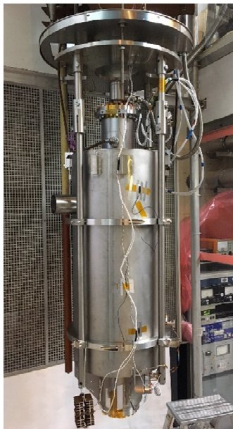
Figure 2: High beta cavity installed in vertical test stand.
