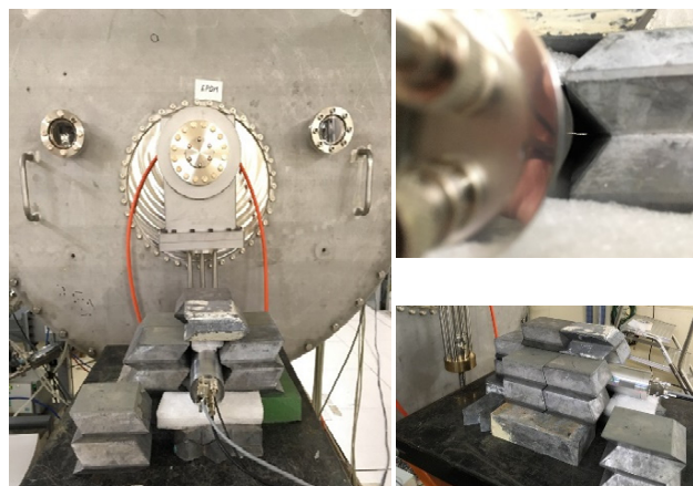
Figure 5: NaI(Tl) scintillator set up during cryomodule test, shielding and collimator aperture are shown respectively on the bottom-left and top-right corner of the figure.
