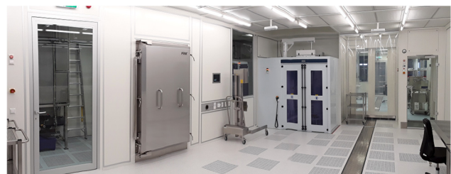
Figure 2: Photo of CR 2 (ISO-4): the HPR with its lever for the movable wand (on top) is shown. The door of the vacuum oven and a lift trolley is shown as well.
