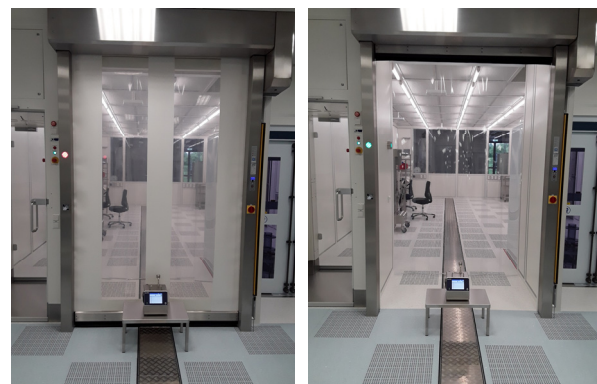
Figure 5: Closed (left) and opened (right) roll-up door with the particle counter placed in front of it in CR 1.
