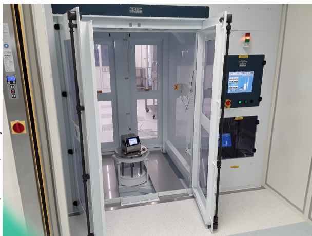
Figure 10: Photo of HPR cabinet with open doors taken from CR 1. A particle counter is placed on the rotating table.
