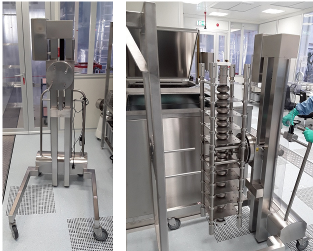
Figure 7: The photo on the left shows the trolley, while on the right the lift trolley during testing of the cleanroom infrastructure with a 3 GHz cavity [21] from TU Darmstadt is depicted; handing over a cavity in its frame to the lifter system of the ultrasonic bath.
