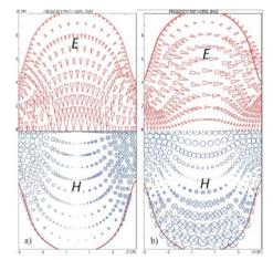
Figure 1: a)  $H_{II0}$  and b)  $E_{II0}$  trapped dipole modes in a single cell TESLA type cavity.
