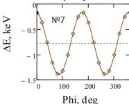
Figure 4: Beam energy depending on RF phase of #7 dipole
