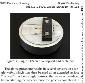
before starting the process; once the process completed, it is easy to cut the wafer into single-sensor portions. A microscopy image of a single sensor is shown on Fig. 1, while a wafer with 30 sensors is shown on Fig. 2 and a single sensor assembled in a circular support is shown on Fig. 3.
