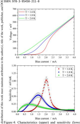
Figure 4: Characteristics (upper) and sensitivity (lower figure) of TES versus bias current, at 3 temperatures.
