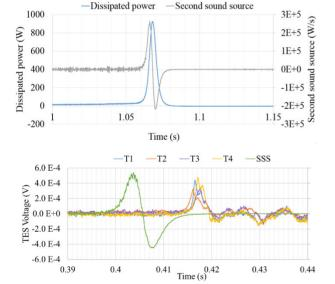
Figure 7: Above: Dissipated power and its time derivative, or second sound source. Below: second sound source signal (green, arb. units) and response of the four TES sensors above the cavity.
