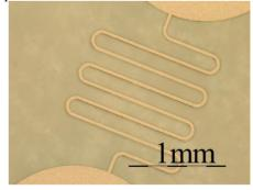
Figure 1: Micro photography of a thin film Transition Edge Sensor with 225 nm Sn on 20 nm Au.
