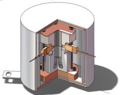
Figure 3: Full assembly with two layers of magnetic shielding, IR shield copper cap, SMA penetrations, and niobium 3D resonator.
