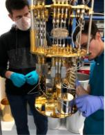
△ Figure 5: 3D QWR assembly (left), attached to the 10mK stage of the dilution refrigerator at the University of Chicago (right).
