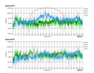
Figure 3: Disturbance from Circulation Pump (upper turn-on, lower - turn-off).
