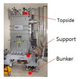
Figure 1: Installed QWR SC Cryomodule.
