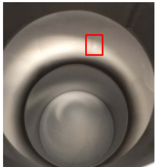
Figure 3: A picture of SC-IB interior after second Nb 3 Sn coating. Note the shiny spot marked by red rectangle.
