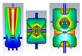
Figure 3: From left to right, RF magnetic field distribution of: Spiral2 QWR, MYRRHA Single Spoke Resonator (SSR) and ESS Double Spoke Resonator (DSR).
