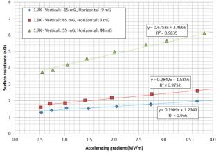
Figure 4: Surface resistance plotted versus accelerating gradient of a Spiral2 QWR for different ambient magnetic field applied: optimal (diamonds), vertical (square) and horizontal (triangle).
