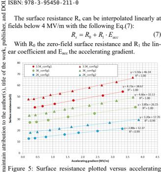
Figure 5: Surface resistance plotted versus accelerating must gradient of a ESS DSR for two different ambient magnetic field applied: low (circle) and high (triangle) and at three work different temperatures: 3.5K, 3K and 2K.
