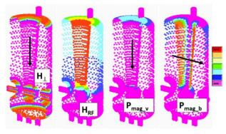
Figure 7: Outputs from Labview routine showing from left to right: the trapped magnetic field  $(H_{\perp})$ , the RF magnetic field distribution  $(H_{RF})$ , the normalized power dissipations caused by trapped flux from vertical  $(P_{mag_v})$  and beam axis  $(P_{mag_b})$  magnetic field for the Spiral2 QWR.
