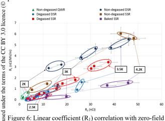
Figure 6: Linear coefficient (R1) correlation with zero-field þ coefficient (R<sub>0</sub>) for Spiral2 QWR (triangle), ESS DSR (cirmay cle) and MYRRHA SSR (square) between 4.2K and 2K and for different heat treatments (10h - 650°C hydrogen work 1 degassing and 48h - 120°C baking).
