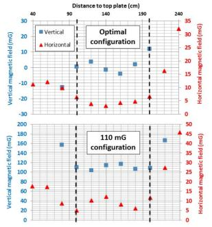
Figure 2: Example of residual magnetic field configuration applied in IPNO vertical cryostat. The vertical and horizontal components are measured along the central axis of the cryostat
