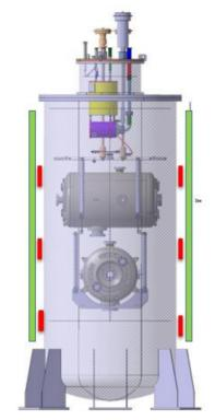
Figure 1: Vertical cryostat in operation at IPNO with its passive and active magnetic shields. The insert is loaded with two ESS Double Spoke Resonators.
