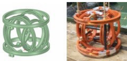
Figure 1: Helmholtz cell formed by 3 paired coils ( \varnothing 110 mm / 96 mm / 76 mm). Left: sketch of the ABS supports. Right: Picture of the assembled coils.
