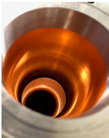
Figure 2: Copper cavity surface after chemical treatment.
