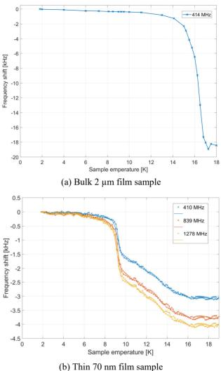
Figure 10: The resonance frequency vs temperature dependence for two samples (*a* and *b*).
