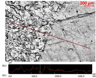
(b) Image from the *Laser Scanning Microscope vk-x200* and surface profile along the red line in  $\mu$ m.
