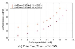
Figure 8: Surface resistance vs B field measurements for two (a and b) samples
