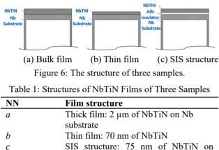
15 nm of AlN insulator on Nb substrate
