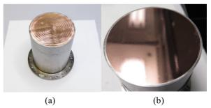
Figure 2: One of the Cu substrates after fabrication (a) and after first SUBU polishing (b) [<sup>©</sup>Credits: Cristian Pira, E. Chyhyrynets and other. INFN LNL].
