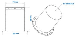
Figure 1: Samples dimensions and shape.
