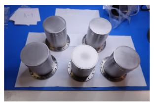
Figure 4: Five Nb substrates after fabrication and mechanical polishing.
