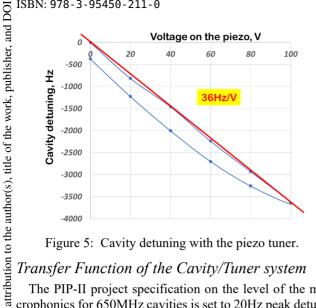
Figure 5: Cavity detuning with the piezo tuner.
