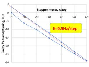
Figure 4: Cavity detuning with slow tuner.
