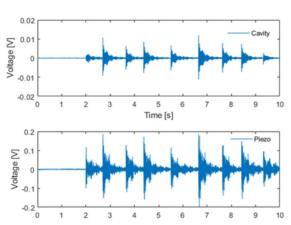
Figure 8: Amplitudes from APD and piezo (as a sensor) when cavity hit with hammer 9 times during 10 second time period.
