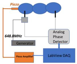
Figure 6: Setup to measure cavity transfer function.
