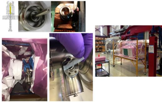
Figure 6: Broken HOM feedthrough replacement.
