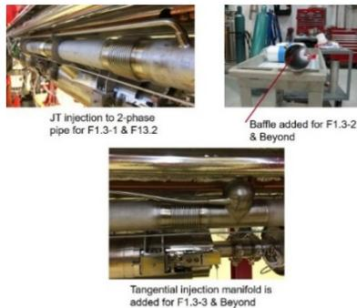
Figure 2: Better Liquid Management and Microphonics Optimization.
