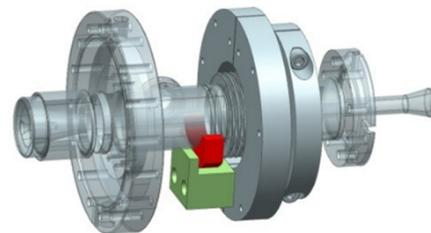
Figure 12: M-mount installed on an LCLS-II coupler.
