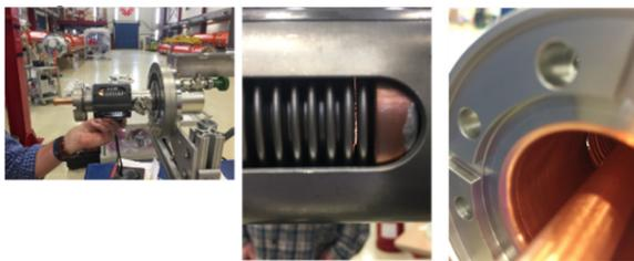
Figure 9: First convolution of the bellows is broken.
