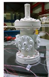
Figure 8: BPM cold shocked tested.
