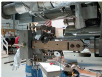
Figure 4: Added bellows between gate valve-Cav#1 and decoupled gate valve support from HGRP to reduce Cav#1 microphonics.
