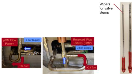
Figure 3: Wipers added to valve stem and reverse configuration welding of the valves to reduce TAO.
