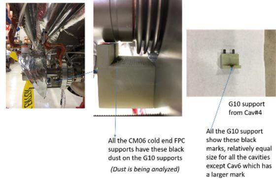
Figure 10: G10 coupler supports friction dust and scoring points to excessive motion during cryomodule shipping.
