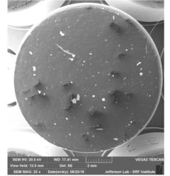
Figure 3: Sampled particulates from girder 1L12 from shaken bellows at location 13 in Fig. 2.
