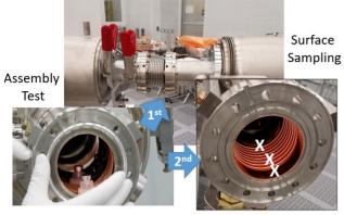
Figure 7: Particulate assessment of LCLS-II bellows assembly.
