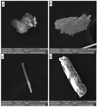
Figure 6: Particulates collected from C100-6 beamline, a) silver, b) copper, c) steel, and d) titanium.
