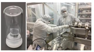
Figure 1: Standard sample spindle and example of particulate sampling from cavity interior.
