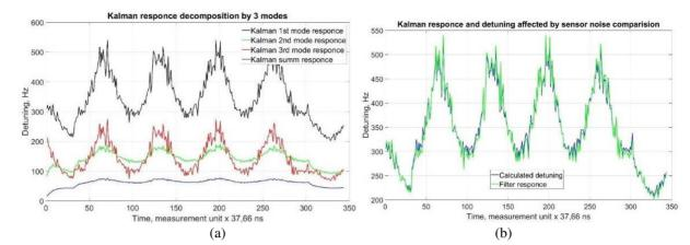
Figure 9: Composition of several mechanical modes of different shape, quality, coupling and noise. (a) shows decomposition of 3 mechanical modes 330, 460 and 470 Hz. (b) shows Kalman filter tracking ability for those mentioned signals.
