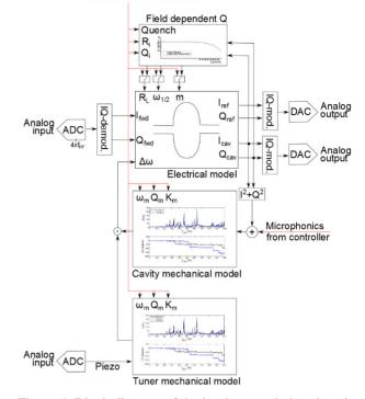
Figure 4: Block diagram of the implemented virtual cavity with the piezo tuner block.
