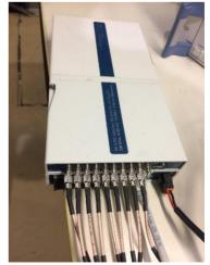
Figure 2: National Instruments NI-7935R FlexRIO controller, [2] with the NI-5783 Analog Adapter Module, [3].
