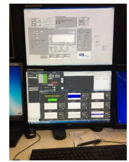
Figure 10: Virtual cavity GUI (above) and LLRF EPICS panels (below) running in the same computer of the control room.
