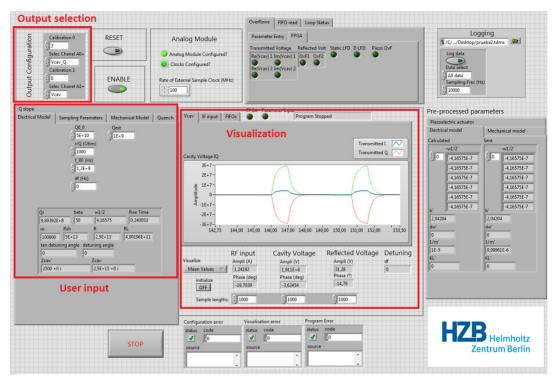
Figure 3: Graphical user interface where the parameter input, analog output selection and data visualization are depicted.
