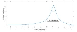
Figure 5: Frequency response of the piezo tuner mechanical block with an eigenmode at 40 Hz with a quality factor of 10.
