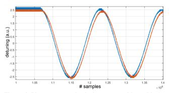
Figure 6: Piezo tuner mechanical response without (blue) and with a 50 ms phase lag (red) with a  $10^{-7}$  s sampling period.
