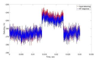
Figure 8: Detuning emulating the real processes of 1 mbar pressure change in LHe system or a non-synchronized beam injection into BESSY-II generated with the virtual cavity (red) and the Kalman filter estimation (blue).
