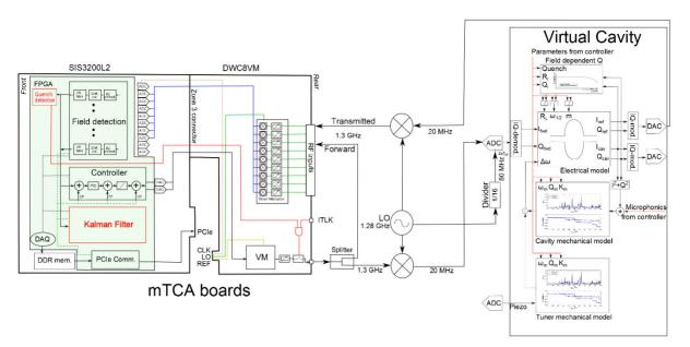
Figure 7: An Up/Downconverter has been used to convert the signals coming to and from the virtual cavity (center of the image) to enable the use of mTCA.4 boards (left).
