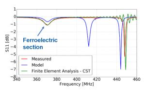
Figure 7: The magnitude of S11 against frequency: measured with the VNA (red); derived from a simplified TLM (blue); and calculated with CST Microwave Studio (green).
