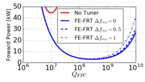
Figure 5: Dependence of forward power on the external Q of the fundamental power coupler for the PERLE 5-cell cavity with and without an FE-FRT. The effect of residual frequency detuning  $\Delta f_{\mu}$  are also shown.
