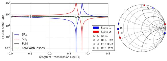
Figure 2: The theoretically derived relations between  $SR_1$ ,  $SR_2$  and the FoM with and without losses for an exemplar FE-FRT model as a function of line length (left) and selected corresponding values of  $\Gamma_1$  and  $\Gamma_2$  (right).
