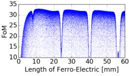
(b) The FoM vs. length of ferroelectric section.
