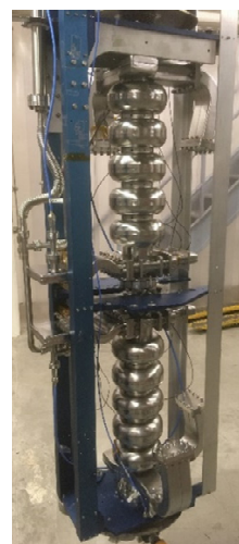
Figure 3: C75 cavity pair attached to a vertical test stand.
