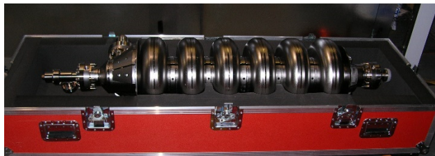
Figure 2: The first cavity (PPU-01) delivered to Jefferson Lab. The cavity was under vacuum with an all-metal right angle valve (left end) and burst disc (right end).
