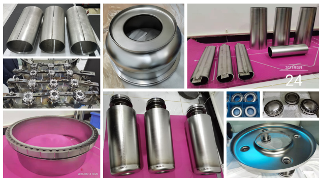
Figure 8: The fabrication of the HOM-damped cavity.
