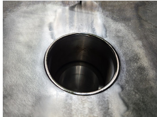
Figure 13: RF port assembly after EBW.
