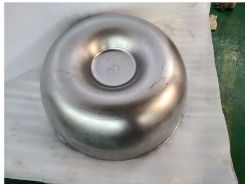
Figure 5: RRR300 niobium press-forming shape.
