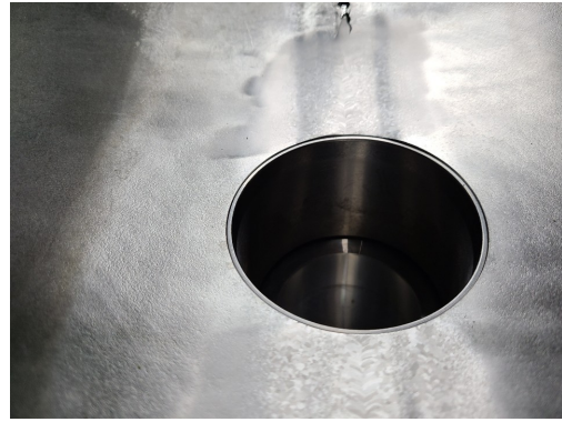
Figure 12: RF port assembly before EBW.
