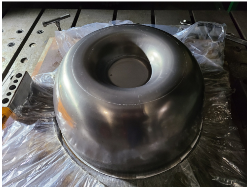
Figure 3: AL6061T0 press-forming shape.
