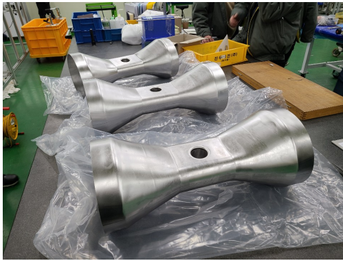
Figure 8: SSR2 Spoke weldment.
