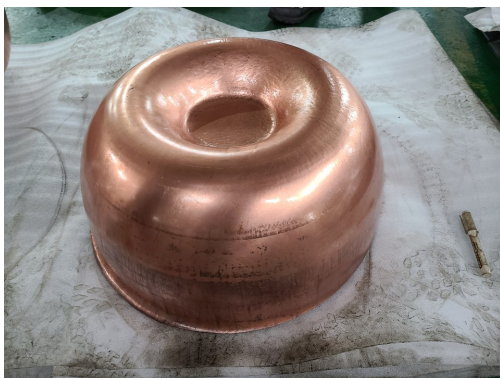
Figure 4: OFHC press-forming shape.
