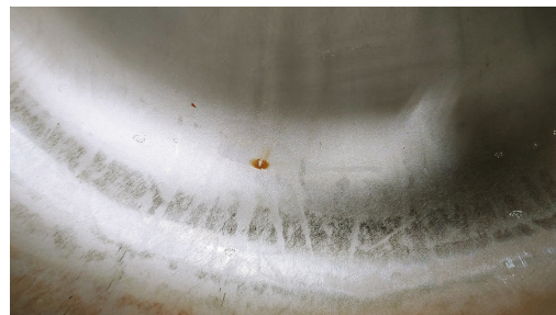
Figure 7: Appeared rust after drying.
