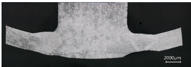
Figure 10: Macrography of welding test sample used to qualify the Nb-Nb hooks' welds.
