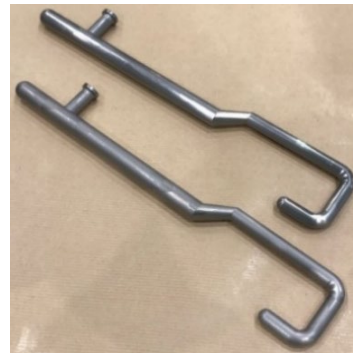
Figure 5: Comparison of surface finishing with two different lubricants: Vascomill™ (top) and Blasocut™ (bottom).
