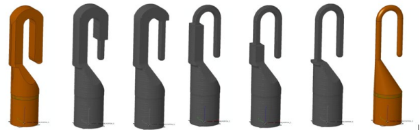
Figure 4: 6-steps incremental machining to obtain the copper hook of the RFD field antenna.
