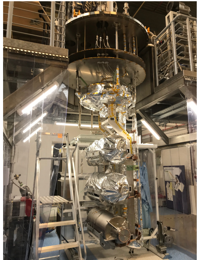
Figure 1: Photograph of CSI on stand with three jacketed cavities installed (top and middle cavities dressed in MLI jackets).
