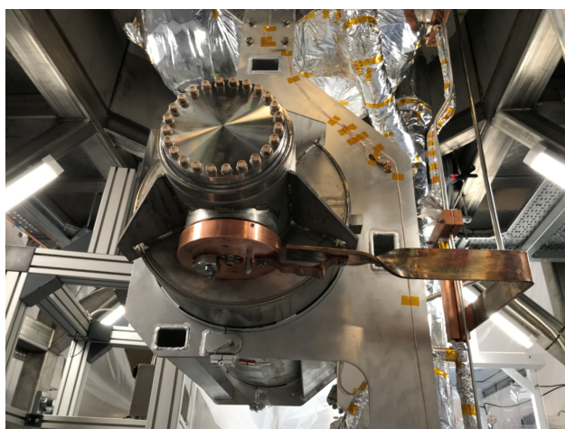
Figure 2: Thermal strap used to provide cooling of the input coupler flange.
