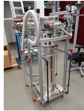
Figure 3: Picture of glass cryostat with two Helmholtz coils producing horizontal magnetic fields and a solenoid wound around the aluminium housing producing field in vertical direction.
