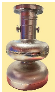
Figure 3: An existing 1.5-cell TESLA shape SRF niobium cavity to be used for the proof-of-principle experiment.
