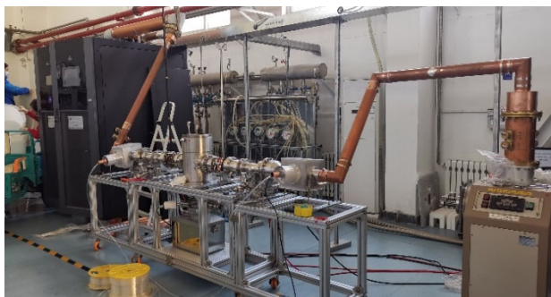
Figure 4: Commissioning test stand of the coupler at IHEP.
