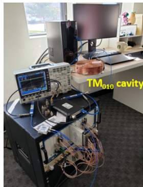
Figure 8: 1.3 GHz room temperature copper resonator.
