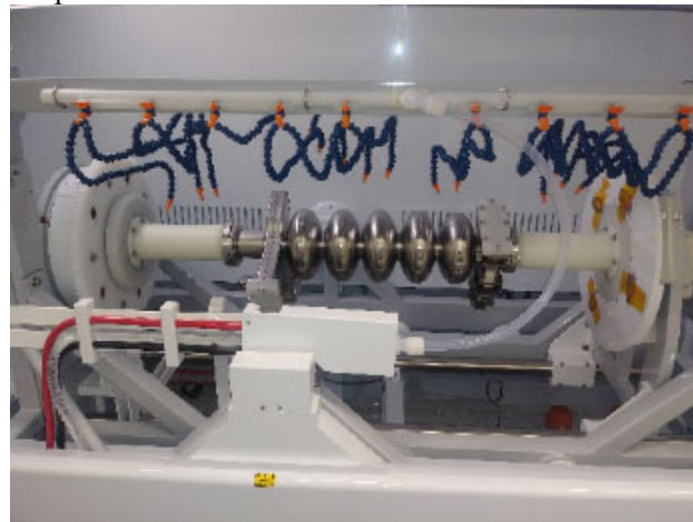
Figure 2: 5-cell CEBAF cavity installed for polishing.
