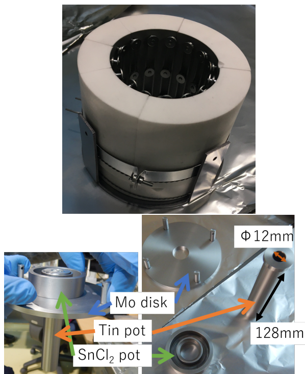
Figure 3: Top: Sn heater. Bottom: Sn crucible and SnCl 2 crucible. Both crucible are made of W.
