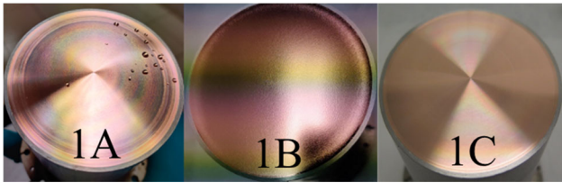
Figure 1: The QPR sample surface. 1A – after non-optimised lathe; 1B – same QPR polished with pitting close to the border; 1C – optimised lathe polishing.
