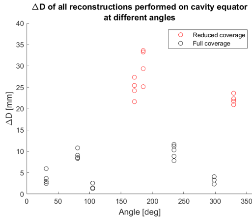
Figure 6: \Delta D -values of all reconstructions performed with calibration tool plotted against the angular coordinate of the resistors true position. Areas with reduced sensor coverage highlighted in red.
