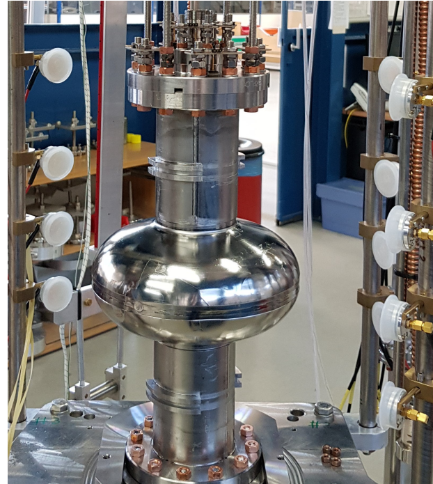
Figure 1: Oscillating superleak transducers (here with white cover caps) mounted on an insert supporting a TESLA-shape single cell SRF cavity with a resonant frequency of 1.3 GHz.
